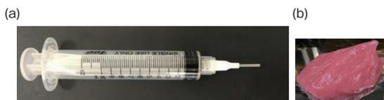
Fig. 1. a) Disposable syringe was filled with (2) paste type food ink, especially with SPI-based ink, in this study, and placed on the paste extruder to automatic extrusion by the designed manner.
