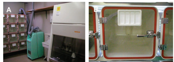
Fig. 2. (A) Safety cabinet used for virus preparation (AIRTECH Japan Ltd.) and B.B.H. Infected Animal Rearing System SEOBiT. (B) B.B.H. Infected Animal Rearing Unit (SEOBiT). Cited from Fig. 1 in Sakudo et al. 6)
